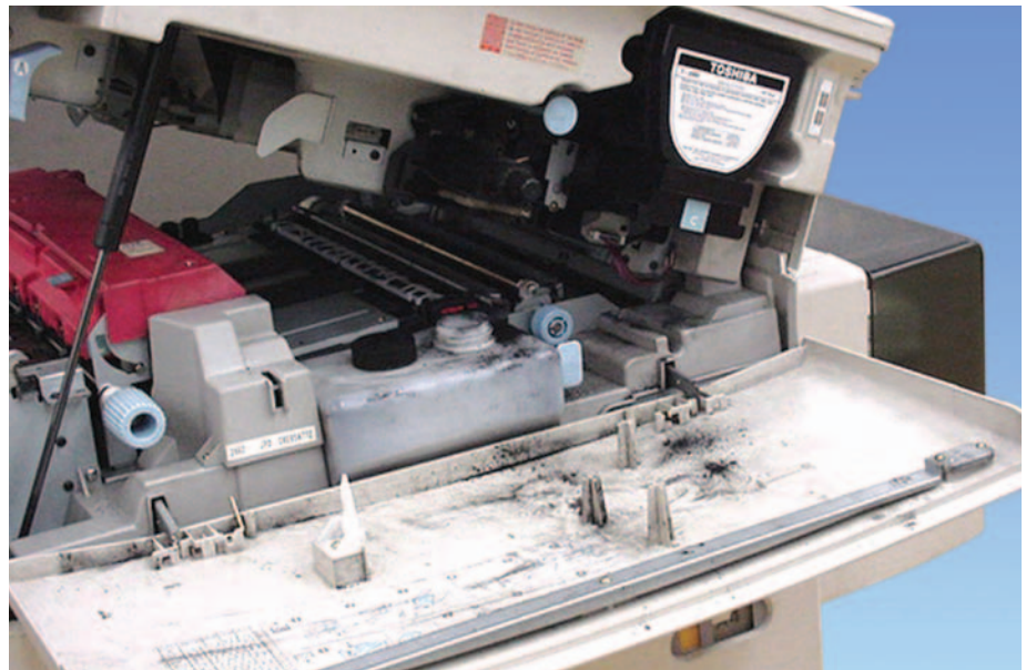
Toner spills due to counterfeit toners reduces overall quality and life span of copier
