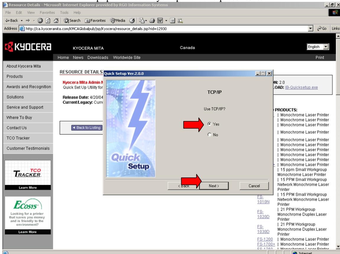
Enter the ip address, subnet and gateway that are to be assigned to the printer. RGO strongly recommends for continued optimal printer performance that a **STATIC ip address** be set for the printer outside the DHCP range. A reservation by MAC address in DHCP is NOT recommended as this method is designed for client reservations. Instances of intermittent loss of printing have been reported in the past due to software issues when dhcp reservations are utilized. Press **Next**.
